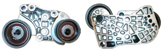
This tensioner/bracket assembly is an indicator that you have a late model system. In this case you will use the YELLOW marks on the belt for the right camshaft and crankshaft during setup.
