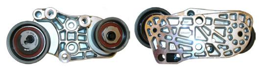
This tensioner/bracket system is an indicator that you have an early model system. In this case you will use the WHITE marks on the belt for the right camshaft and crankshaft during setup.
